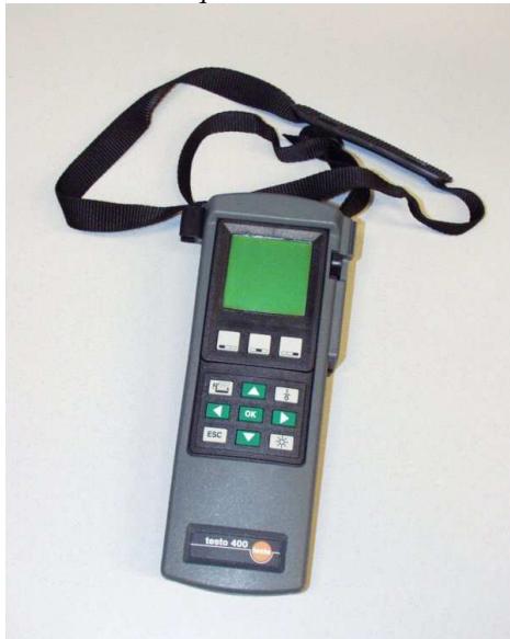
Fig. 10, testo400 handheld datalogger.
